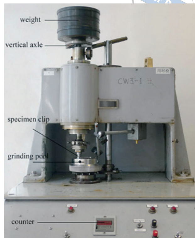
Fig 1 The CW3-1 wear machine.
